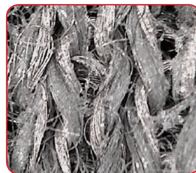
Microscopic view of Carraro Conductive Suit with helically wound silver yarn (shiny silver) in comfortable knit fabric.
