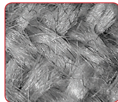
Microscopic view of a typical suit using stainless steel fibers (black strands) in a woven fabric.
